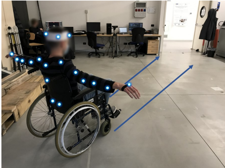
Figure 100. Passive markers disposition on human body during the movements acquisition.
