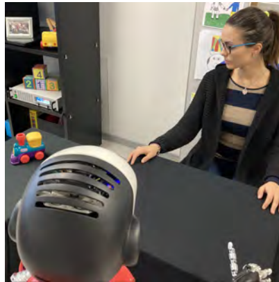
Figure 2.4 Integration of the other's attention. An example of human-robot joint attention elicited by the human. The robot's attention is attracted by the other's attention and is brought to detect the toy train on the table.
