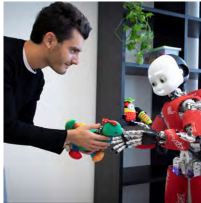
Figure 2.6 Integration of the other's action. An example of how the action of others can be integrated and used to perceive an object. The human is giving the stuffed green dragon gently and carefully to the robot, with two hands. A robot endowed with social perceptual abilities should perceive the stuffed dragon as something delicate or precious and, accordingly, use two hands to handle it.
