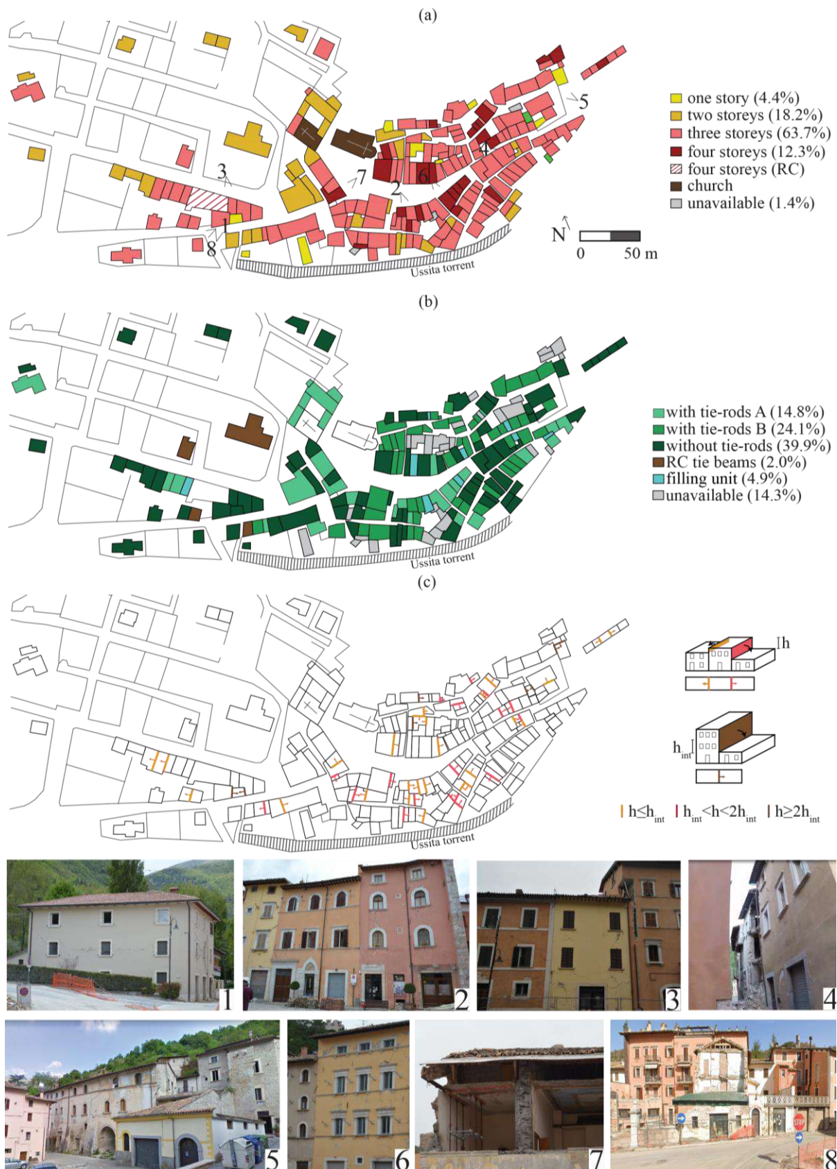
Figure 5.3. Collection of data in the historical center of Visso in terms of: (a) number of storeys; (b) structural details and (c) soaring portions (i.e. in elevation irregularity). (d) Photos of typical buildings in aggregate present in Visso's municipality.
