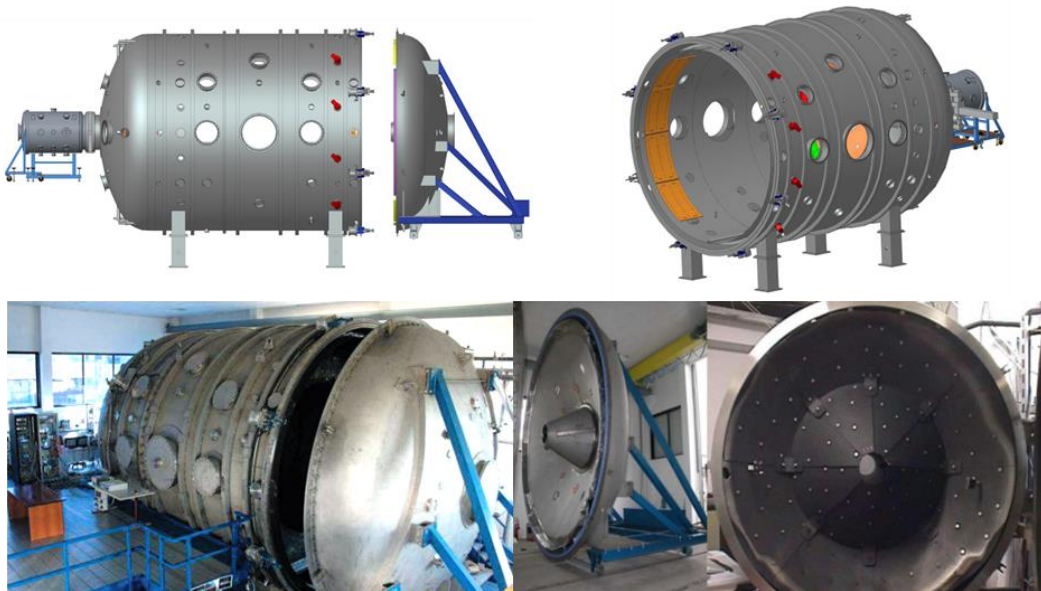
Figure 106: (Top picture) IV10 vacuum facility rendering; (Bottom-Left) IV10 laboratory and (Bottom-Right) movable cap equipped with conical Grafoil targets (credits: SITAEL).
