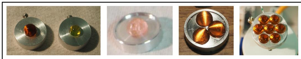
Figure 3.26 – Top: example of commercial PAAm hydrogels initially tested, containing perfumes (1, 2, 3) and water (4), respectively. On the right, two examples of molecules used as smell enhancer in the 1-3 hydrogels. Bottom: examples of the lower electrodes with cavities for holding the hydrogels.
