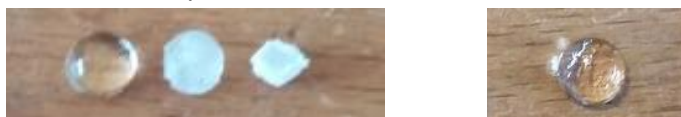
Figure 3.30 – On the left, three PAAm hydrogels at different times after being extracted from KCl 0.5 M (at 60°). From left to right, hydrogel as extracted from solution, hydrogel 3 hours from extraction, hydrogel 3 days from extraction. On the right, hydrogel swollen in 6.5 M LiCl solution at 60°C, 5 days after extraction.
