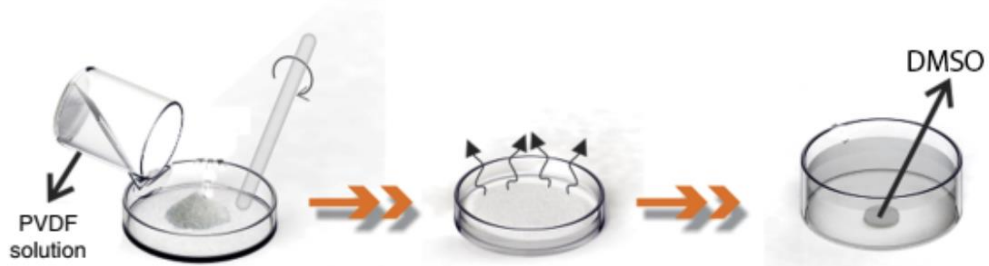
Figure 4.4 – Schematics of the drop casting method, here for a solution of PVDF in DMSO [104].
