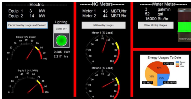
Figure 2.1: A dashboard designed using gauges, a light indicator, alternating stoplights, a pie chart, and tables. (NG stands for natural gas) [67]
