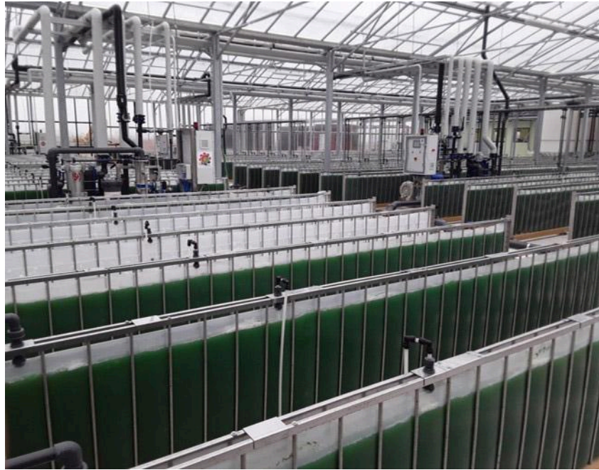
Figure 29 The GWP®-II is a low-cost photobioreactor suitable for pilot plants and commercial installations at the Archimede Ricerche Production site.
