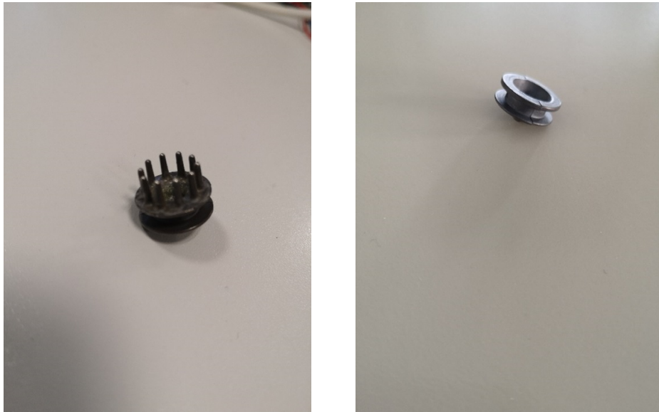
Figure 2.6: The dry (left) and gel (right) electrode
