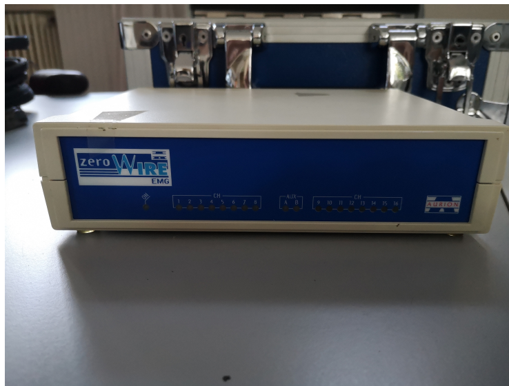
Figure 2.10: EMG device to connect sensor to a PC
