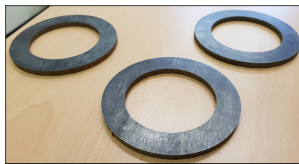
Fig. 3.7 Second set of ARMCO ® Pure Iron specimens to be tested
