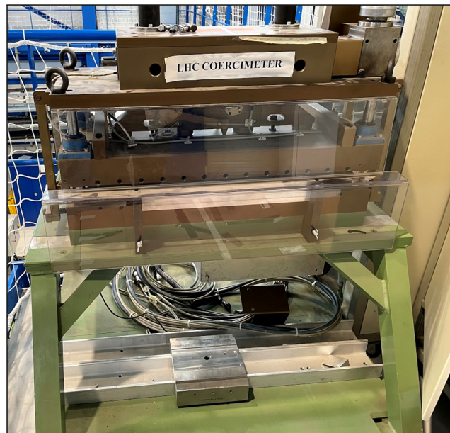
Fig. 2.9 A photograph of the coercimeter, the single-sheet tester used in the past at CERN.
