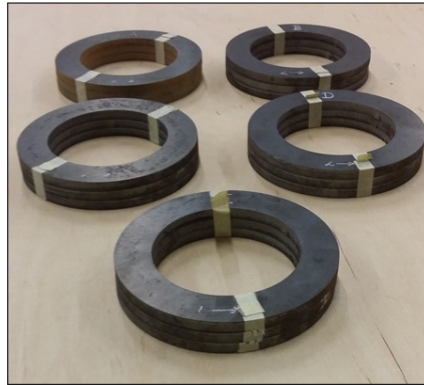
Fig. 3.1 First set of ARMCO ® Pure Iron specimens to be tested
