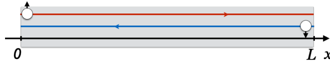
Figure 1.21: Single edge of a two-dimensional topological insulator, hosting two counter-propagating modes with opposite spin.
