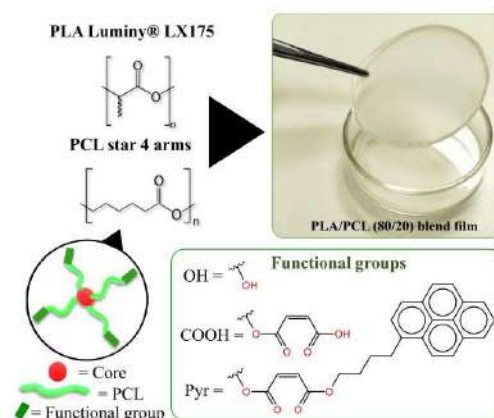
Fig. 1. Scheme of blend film preparation.
