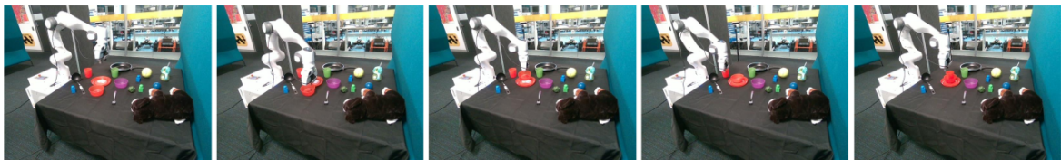
Figure 14.3 Sub-tasks decomposition of a sequence from the Place the bowl on the plate and the cup in the bowl matching the color task.
