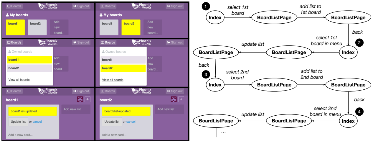
Figure 6.1: Phoenix Trello example and generated crawling trace containing dependent and redundant test cases.
