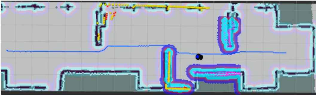
Fig. 3.7 Test Case 2: OSGP behaviour when a human obstacle is sufficiently far from the AMR.
