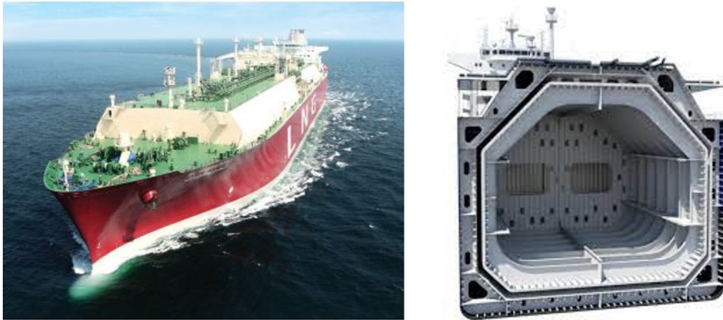
Fig. 4.4 LNG carrier (left) and its corresponding membrane containment system (right) [14, 15].
