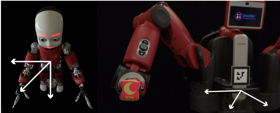
Figure 7.4 Robots' movements direction: the three planes along which the motions were generated, namely frontal, sagittal and oblique with respect to the robots' reference frame, are marked with white arrows.
