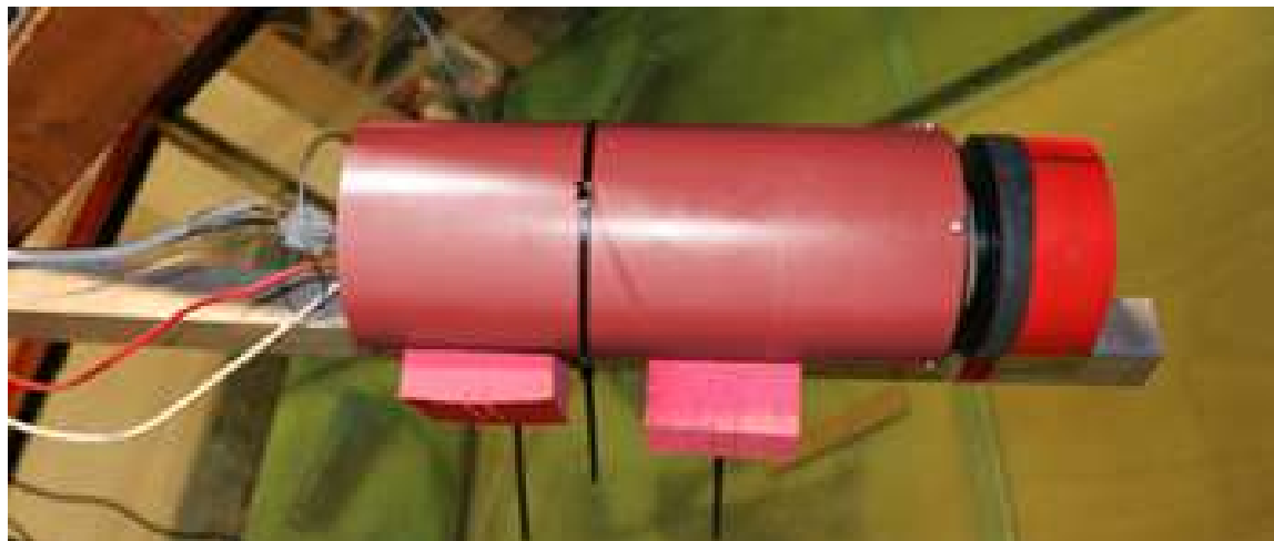
Figure 5.36: The Pump-Jet Module prepared for the testing phase.
