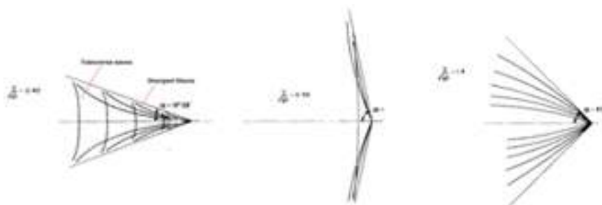
Figure 4.19: The wave formation in shallow water depending on Fn_H [140]
