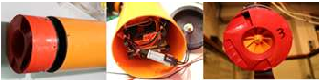
Figure 5.26: The Pump-Jet Module final layout
