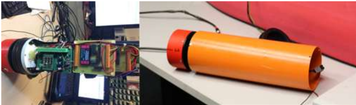
Figure 6.4: The assembly of the Pump-Jet Module
