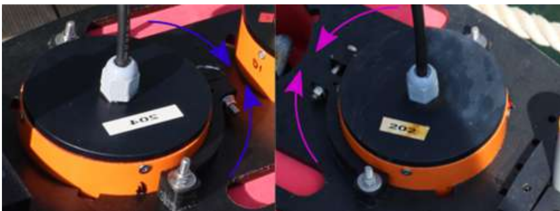
Figure 7.3: The clamp for blocking the motor's rotation
