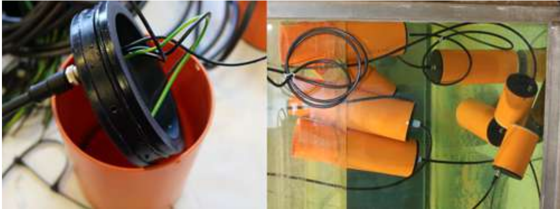
Figure 7.1: SWAMP elements water pressure tested
