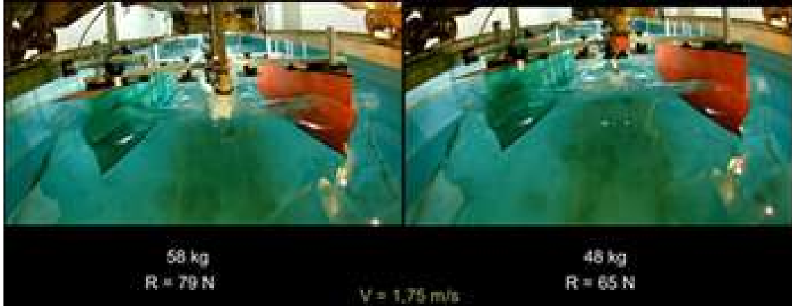
Figure 4.26: SWAMP in the towing tank facility during high speed tests
