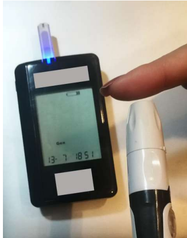
Fig. 1.4 Glucometer with pen blood lancet and test strip. A drop of blood, collected by pricking the finger with the lancet, is spilled on a disposable test strip and then analyzed by the device. Finally, the device displays the blood glucose level in units of mg/dL or mmol/L [1].
