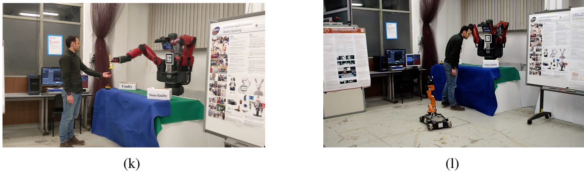
Figure 4.6 Different stages of the Human-Robot Collaboration in which the operator alters the execution of the plan online.
