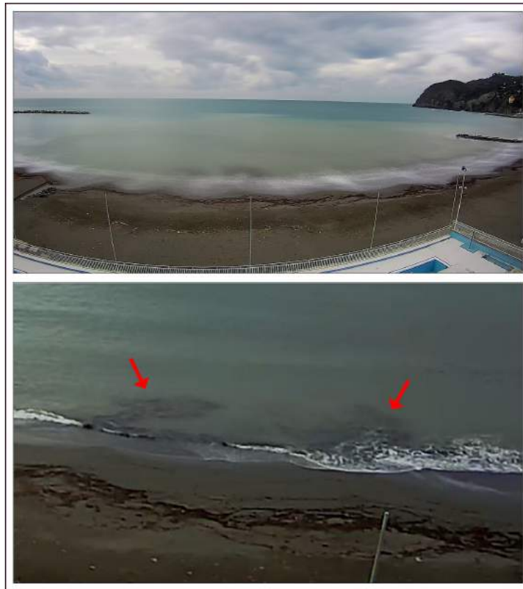
Figure 5.7: Rips associated with cuspidate morphologies along the beach eastern sector (central camera). (Top panel) timex image. (Bottom panel) rip details (zoomed snapshot).
