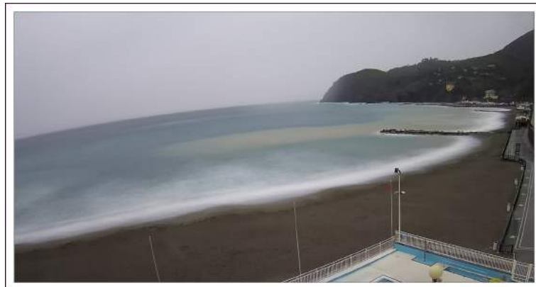
Figure 5.3: Rip current development on the west side of the groyne (timex image). Rip behaviour is traced by water turbidity.
