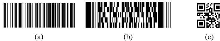
Fig. 6.1 Barcode technology evolution: a) Code 128. b) Code PDF417 and c) QR Code.
