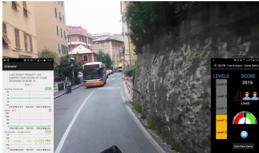
Figure 32: in-vehicle smartphone-based evaluator transmitting scores to driver game scene on test drive in public bus-Genova
