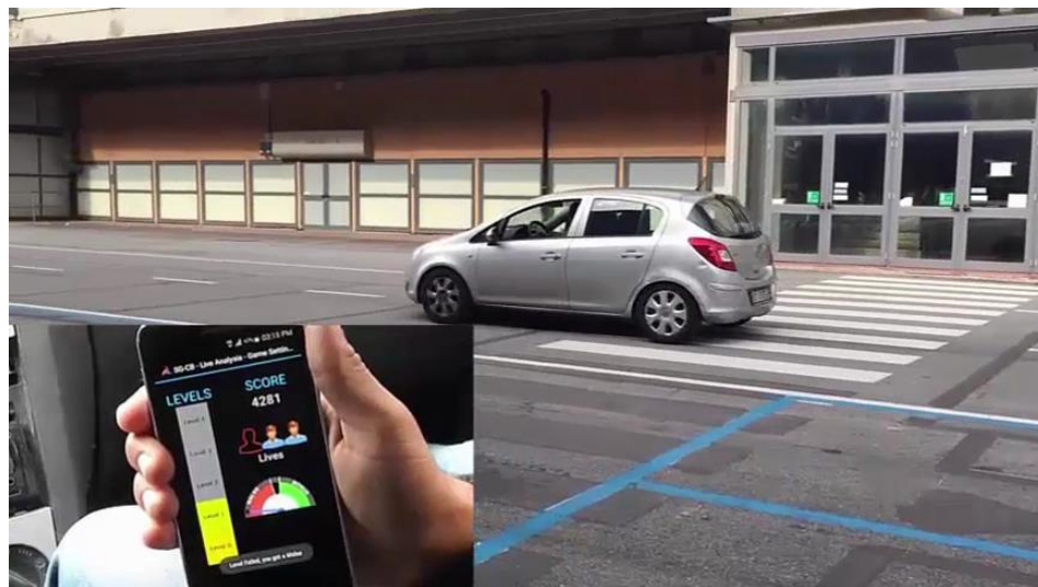
Figure 36: Driver game scene indicating the impact of poor driving performance - the picture from driving session while the driver was exhibiting harsh brakes
