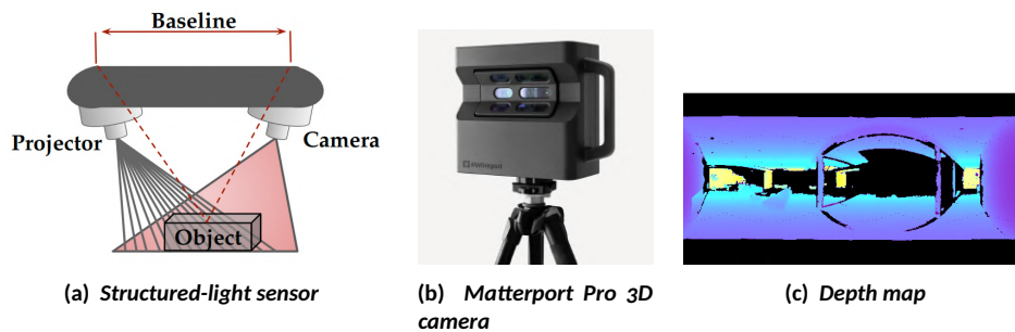
Figure 2.5: Structured light scanners. Structured light scanners use trigonometric triangulation by a projector to display a series of linear patterns onto an object. Then, by analyzing the distortions of these lines or dots is determined the depth, Fig. 2.5a. Although, the captures can have some artifacts such as lots of missing areas when has a large depth as Fig. 2.5c shows, which is a depth map captured by structured-light sensor (Matterport Pro 3D camera, Fig. 2.5b).
