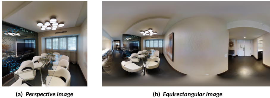
Figure 2.1: Comparing conventional perspective capture with 360° capture. Fig. 2.1a shows a perspective image that is a transformation from the equirectangular image, Fig. 2.1b. Both images are from the Matterport3D dataset [6].
