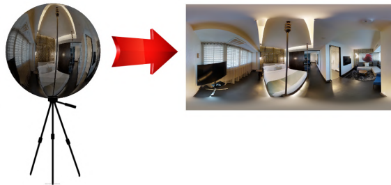
Figure 2.14: Equirectangular image aligned to the gravity vector. Camera is aligned with an horizontal-ground plane.
