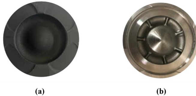
Figure 4–42: (a) Conventional steel-forged re-entrant bowl; (b) hybrid bowl steel-based AM prototype. Adapted from [42].
