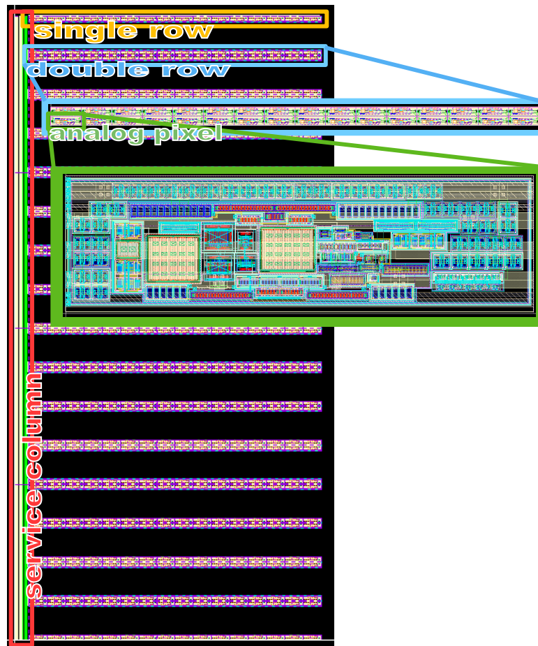
Figure 5.14: Floor-plan of the Timespot1 analog matrix. The most relevant blocks are highlighted. The two single-rows can be seen at the top and bottom of the matrix. The digital-matrix is complementary to the analog one and occupies the block space.
