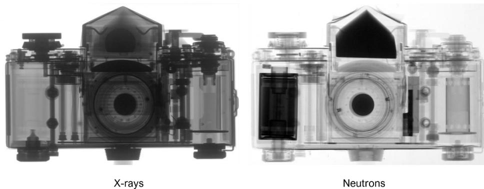
Figure 5.25: Differences in radiograph of an analog camera by X-rays (left) and neutrons (right) (from https://www.psi.ch/en/science )
