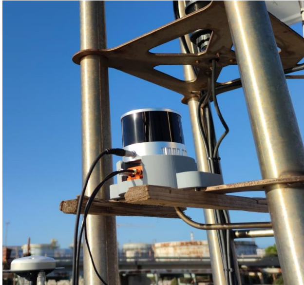
Figure 48. LiDAR and IMU mounting platform setup
