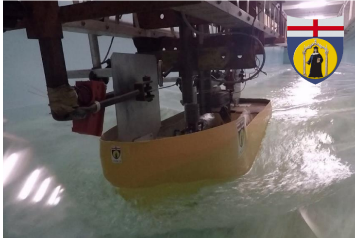
Figure 18: Towing tank test capture
