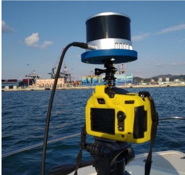
Figure 51. Camera and LiDAR experimental setup
