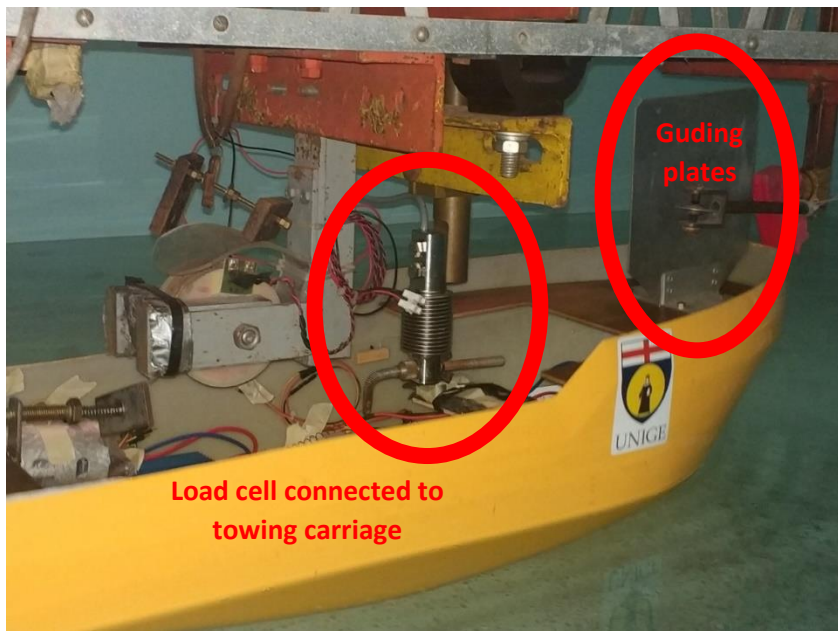
Figure 14. Hull outfitting for towing tests
