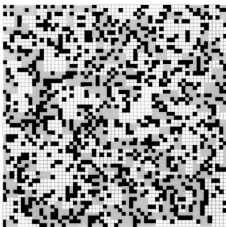
Figure 1.4: Two-dimensional wet cathode structure obtained via stochastic approach. (■) electrocatalyst particle, (□) electrolyte, (□) pore [2].
