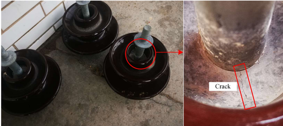
Figure 5-24 Picture of the insulator with a crack.
