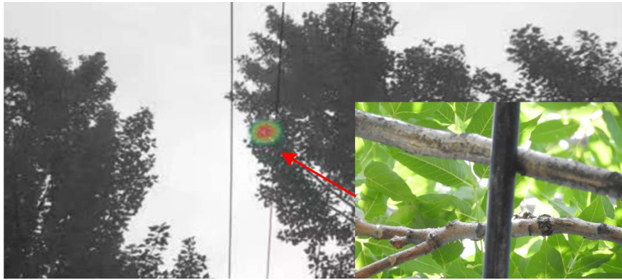
Figure 5-22 Ultrasonic imaging captured using a commercial ultrasonic camera and an inset showing a picture of the tree leaning on the CC line.
