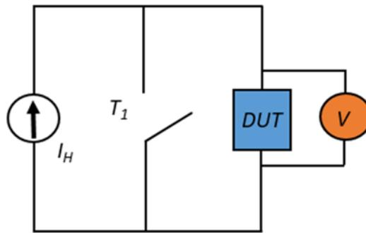
Figure 4:3. Electrical circuits of a DUT for the static measurement of the voltage under high current.
