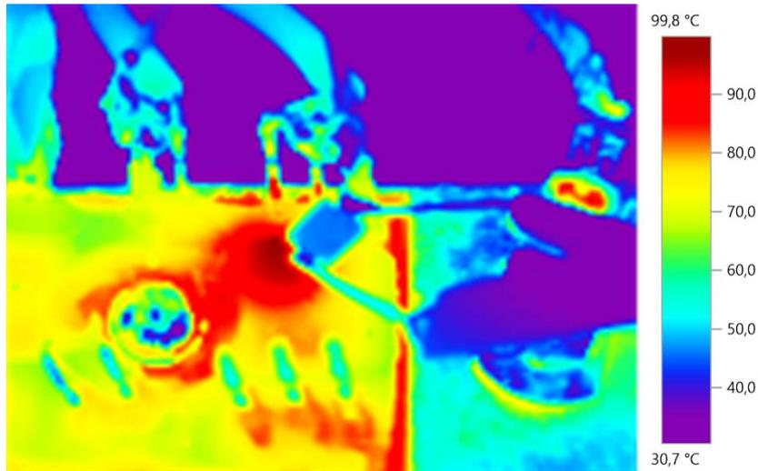
Figure 4:1 Thermal map of a SiC power module in case of current injection in the body diode.
