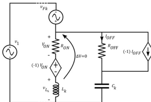
Figure 3:11 A VCVS and a CCCS used to emulate, respectively, a short circuit and an open circuit when  $L_k$  is selected (that is  $d=1$ , then  $L_k$  is connected in the lamp model while  $C_k$  is disconnected).
