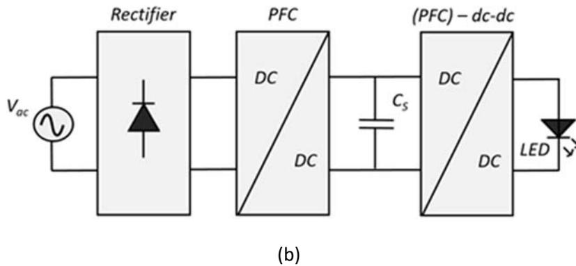
Figure 1:3 (a) SS switching LED driver topology. (b) TS switching LED driver topology.
