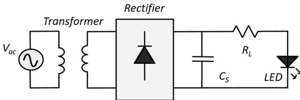
Figure 1:1 Typical application of a passive "lossy" LED driver.
