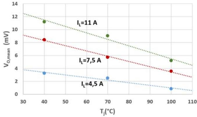
Figure 5:8 Dependence of  $V_{OM}$  with  $T_j$  and  $I_L$  at 3 kHz.
