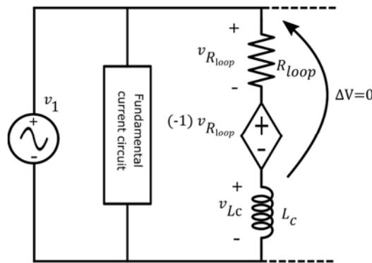
Figure 3:10 VCCS that nullifies the effect of  $R_{loop}$ , thus obtaining a Pspice circuit that actually implements the proposed model.
