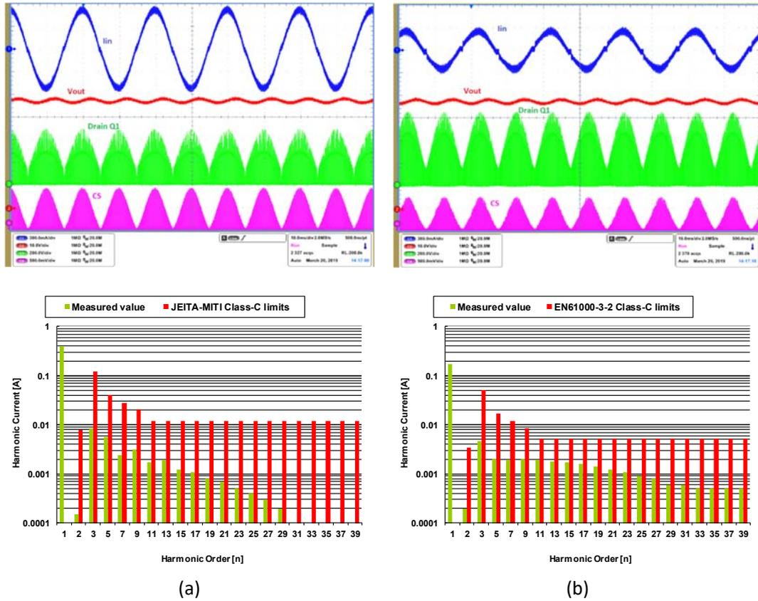
Figure 2:3 Steady-state waveforms at full-load: (a)  $V_{in} = 110\text{ V}$  at  $60\text{ Hz}$ . (b)  $V_{in} = 230\text{ V}$  at  $50\text{ Hz}$ . They have been overlapped by the harmonic contributions of the input current (green bars) with the Japanese norm JEITA\_MITI Class-C (a), and European norm EN61000-3-2 Class-C (b) for lighting equipment.
