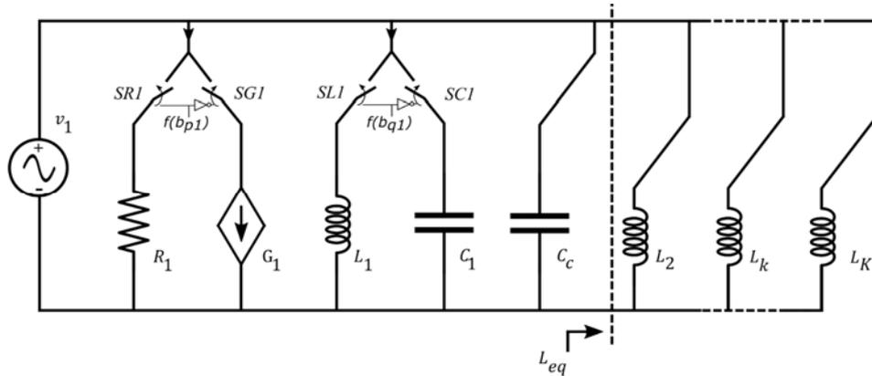
Figure 3:7 Equivalent circuit when only  $v_1$  works while the other independent generators are turned off. It is apparent that a current at the fundamental frequency flows through  $L_{eq}$ .  $C_c$  is thus accorded to nullify the fundamental current downstream from the “fundamental current circuit”.
