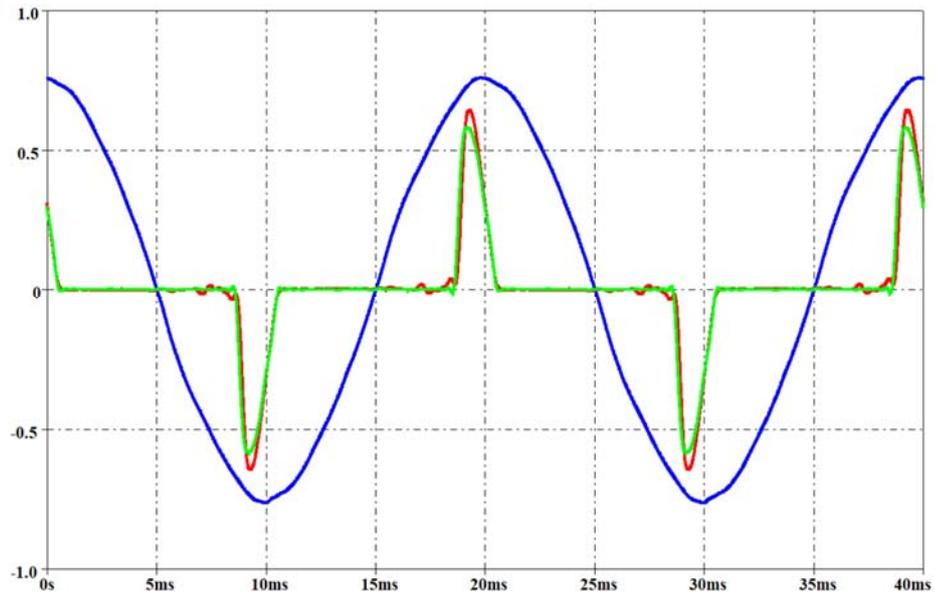
Figure 3:17 Measured voltage on the mains (blue waveform, *rms* 212V), measured current (green waveform), and simulated current (red waveform) for a LED. Per-unit system: base voltage 400V, base current 300mA.
