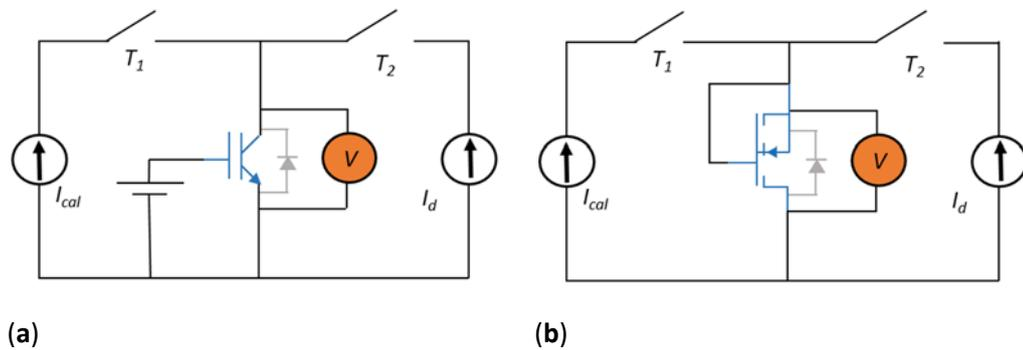
Figure 4:2 Electrical circuits for the static measurement of the voltage under a low current: (a) IGBT (b) MOSFET.
