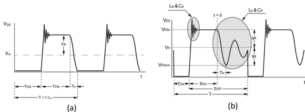
Figure 1:6 Drain to source voltage waveforms for a DCM flyback (a) and a QR flyback (b).
