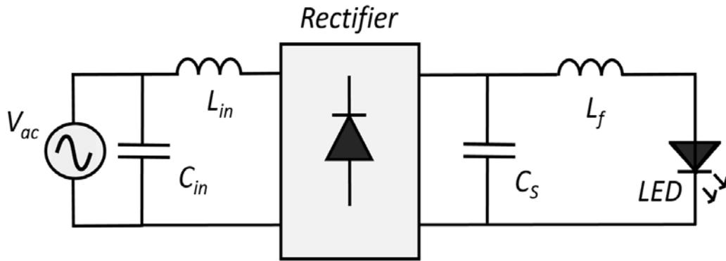
Figure 1:2 Typical application of a passive “lossless” LED driver.
