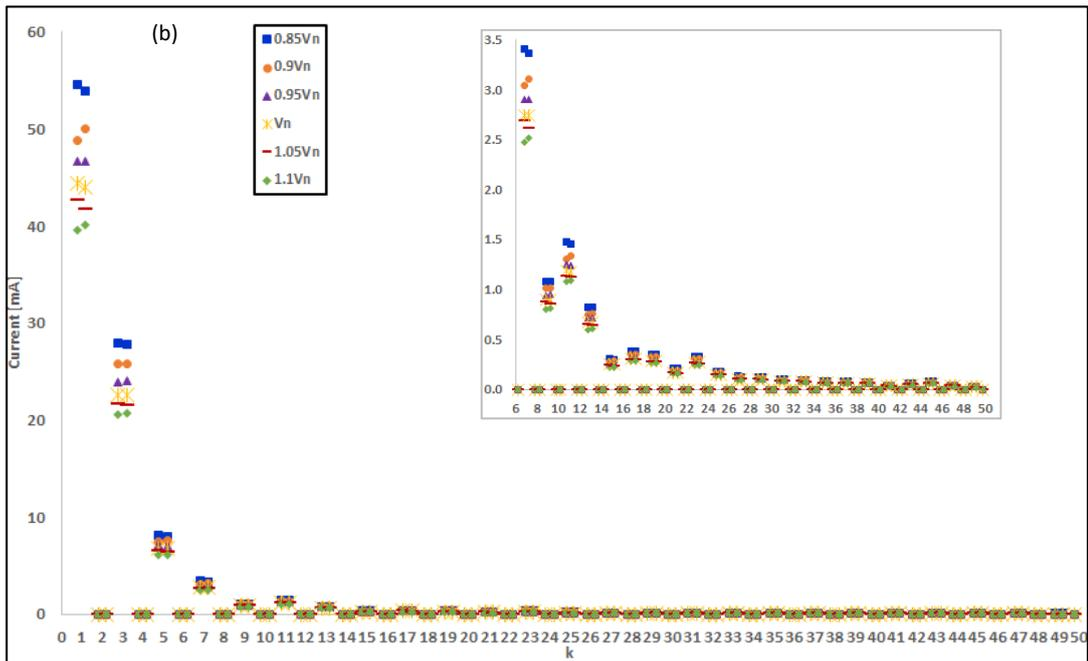
Figure 3:27 Fundamental and harmonics currents obtained by measurements (left) and simulation (right) at six voltage values for LED1 (a) and LED2(b). The sub-figure at the left corner presents a magnification to better observe higher-order harmonics amplitude.
