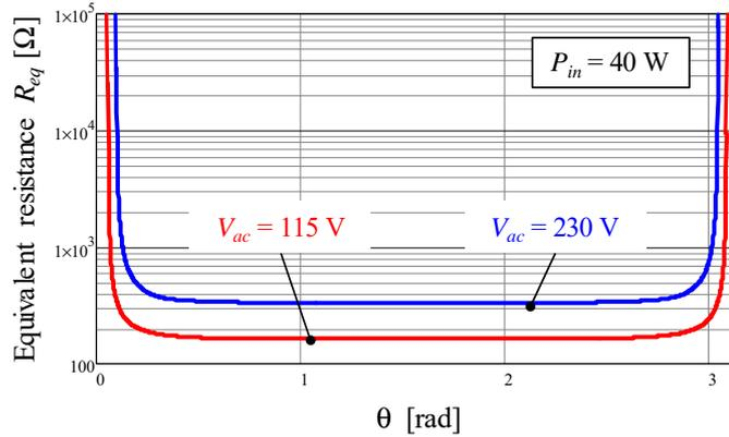
Figure 2:6 Variation of  $R_{eq}(\theta)$  along the sinusoid for the prototype converter caused by the ringing current.
