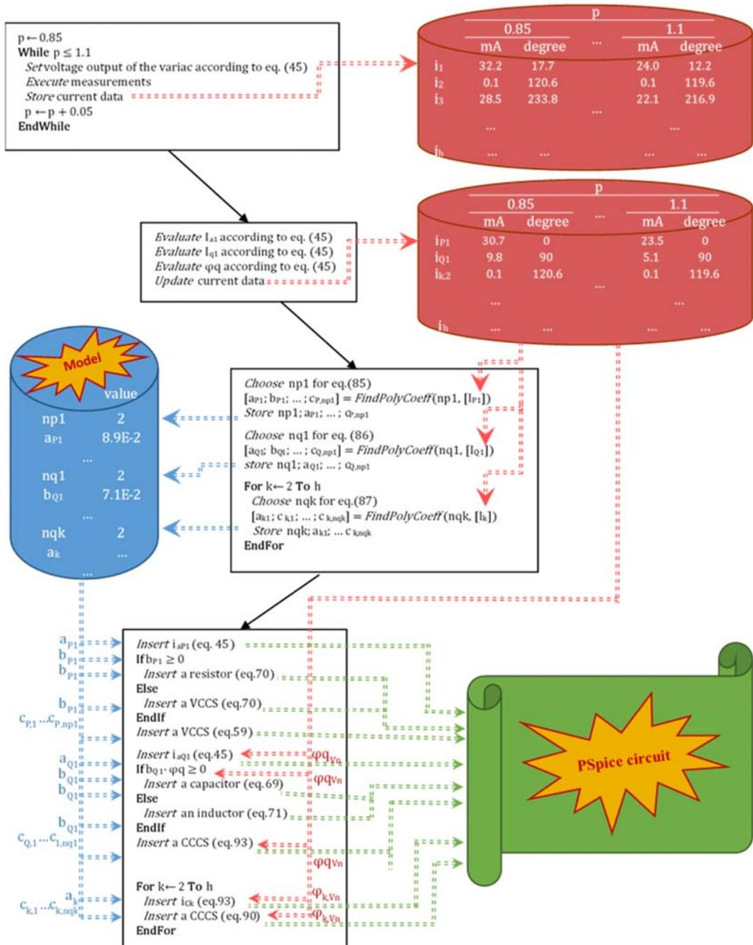
Figure 3:24 Main steps to obtain the circuit model for any LED light bulb using only measurements at its terminal (i.e. black-box model).
