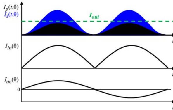
Figure 2:2 Current waveforms of the circuit in Figure 1:7: line cycle time scale of the primary current  $I_p$ , the secondary current  $I_s$ , input rectified current  $I_{in}$  and current in the ac side  $I_{ac}$ .
