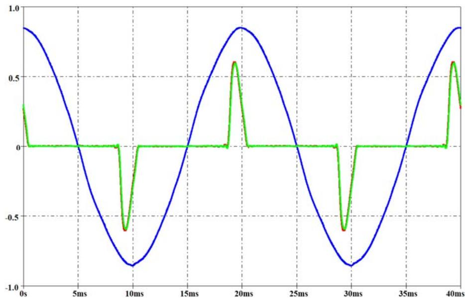
Figure 3:18 Measured voltage on the mains (blue waveform, *rms* 237V), measured current (green waveform) and simulated current (red waveform) for a LED. Per-unit system: base voltage 400V, base current 300mA.
