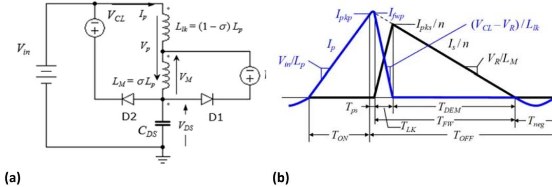
Figure 2:7 (a) Simplified equivalent circuit during off time. (b) Current in the real primary windings (blue trace) and the secondary windings (black trace).
