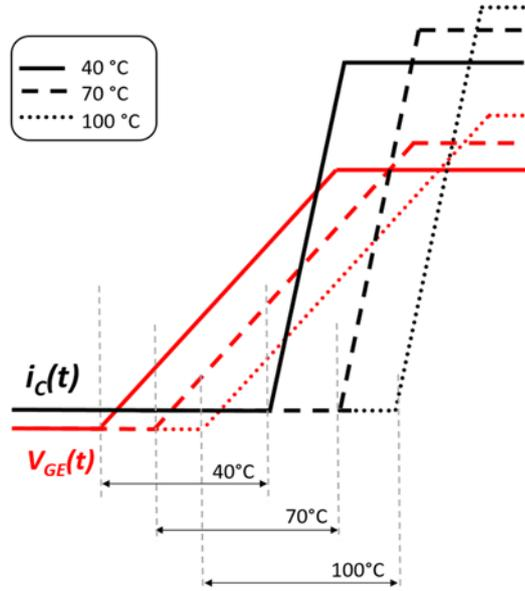
Figure 4:7 Simplified  $i_c - V_{ge}$  turn ON waveforms of an IGBT at different temperature working operations.
