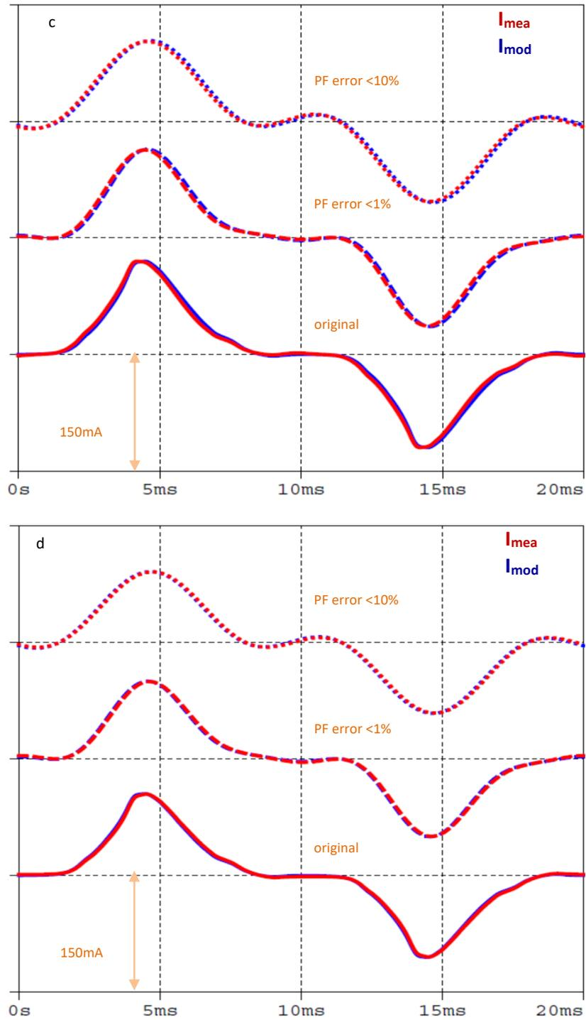
Figure 3:28 Total current drawn by the lamps.  $I_{mea}$  is the measured current (red trace) while  $I_{mod}$  is the simulated current (blue trace):
