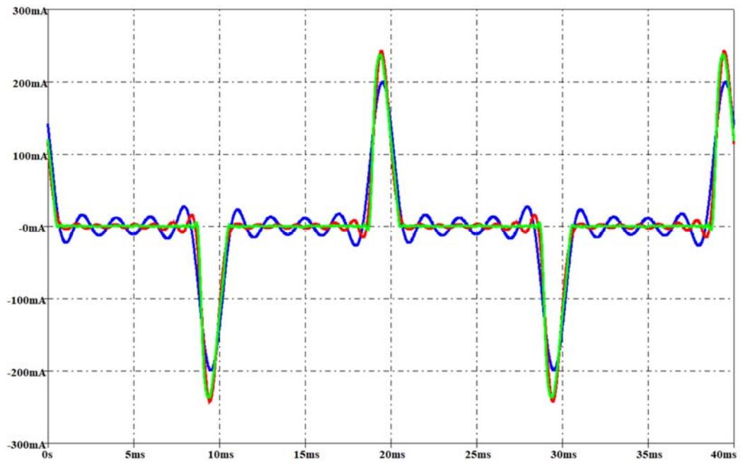
Figure 3:20 LED light bulb: measured current (green waveform) and the simulated current involving a THD error of 1% (red waveform) and 10% (blue waveform) with a rms voltage of 237V.
