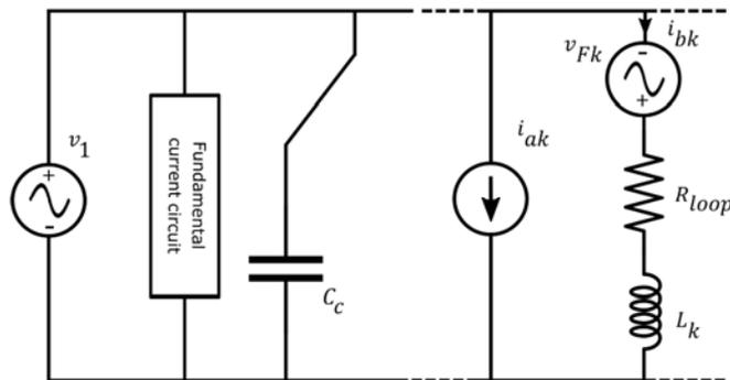
Figure 3:8 Resistance Rloop not belonging to the proposed model but necessary to enable PSpice simulation.
