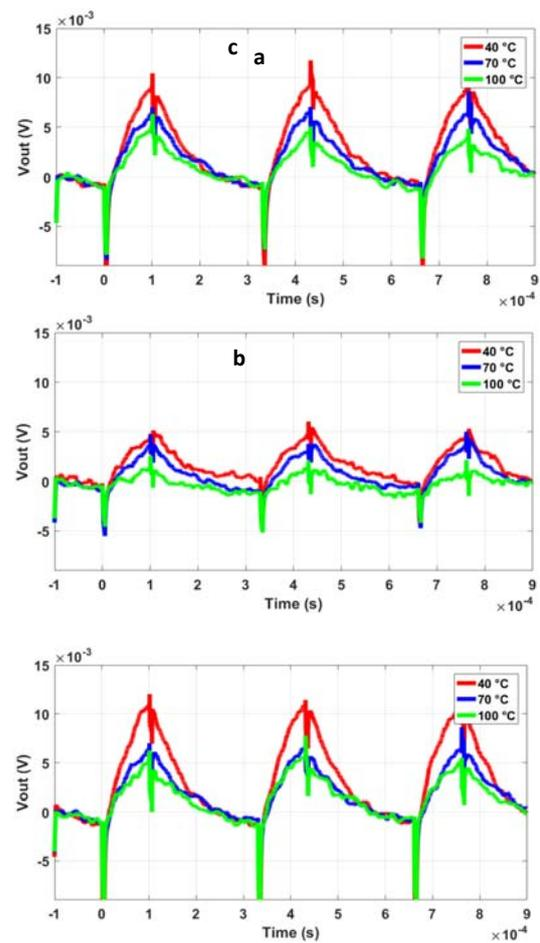
Figure 5:5 Photodiode voltage output at different  $T_j$  and different diode forward current values: (a)  $I_L = 4,5A$  (b)  $I_L = 7,5 A$  (c)  $I_L = 11,5 A$ .
