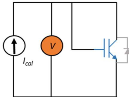
Figure 4:5 Circuit for the calibration step of the threshold voltage method.
