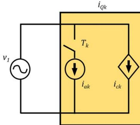
Figure 3:23 Equivalent circuit of the k-th nonactive current harmonic.
