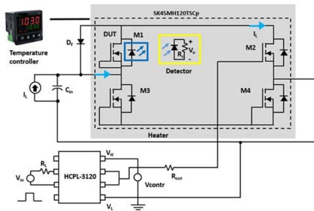
Figure 5:2 Experimental setup schematic.
