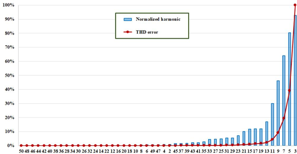
Figure 3:3 Normalized current harmonics and THD error, when the LED light bulb is feed with 212V.
