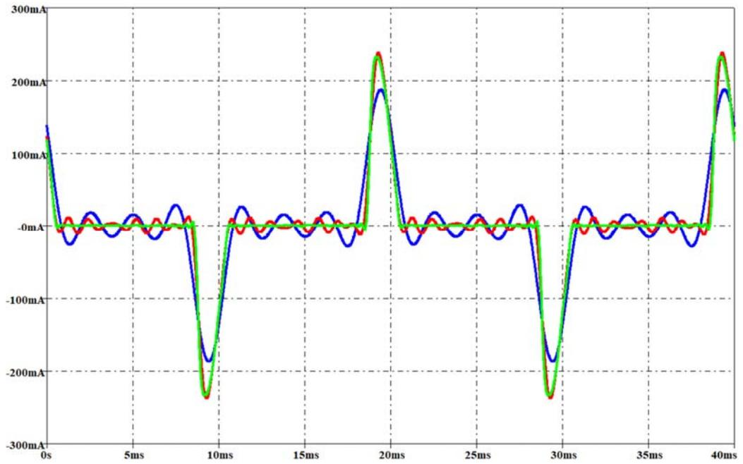
Figure 3:19 LED light bulb: measured current (green waveform) and the simulated current involving a THD error of 1% (red waveform) and 10% (blue waveform) with a rms voltage of 212V.
