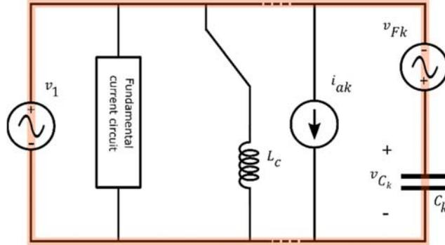
Figure 3:9 KVL for obtaining the voltage across a capacitor adopted in the k-th harmonic circuit.
