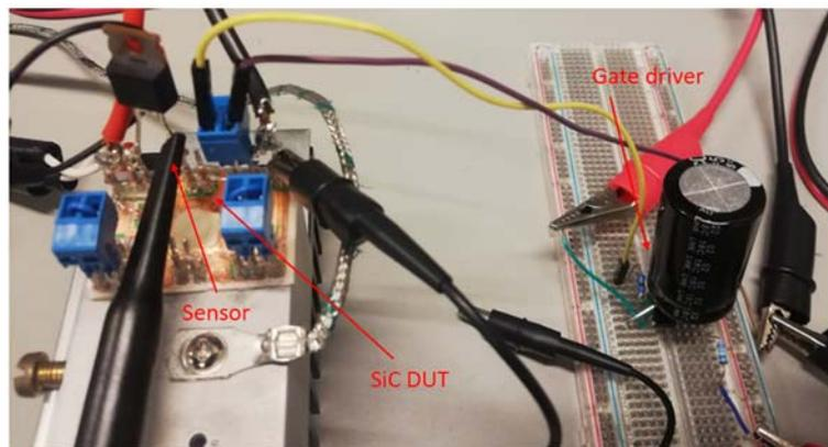
Figure 5:3 Picture of the experimental setup.
