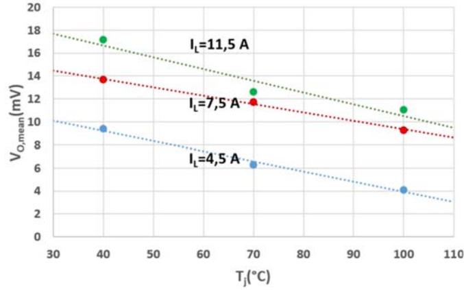
Figure 5:7 Dependence of  $V_{OM}$  with  $T_j$  and  $I_L$  at 333 Hz.
