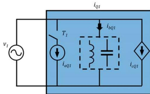
Figure 3:22 Equivalent circuit for the fundamental nonactive current. Only one element in the dashed box has to be used (it depends on the sign of  $b_{Q1}$ ).
