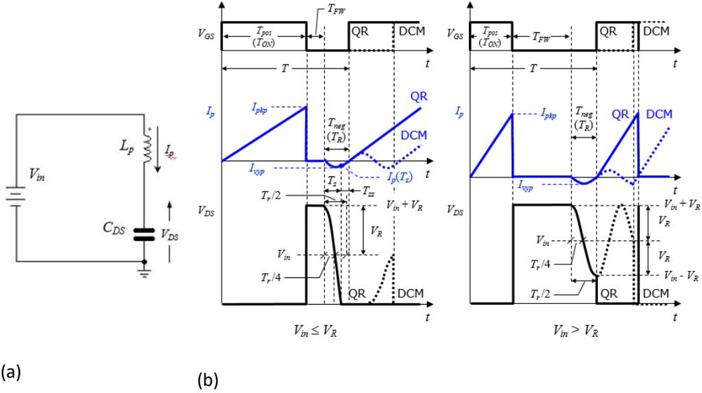
Figure 2:4 (a) Simplified equivalent circuit during  $T_{neg}$ , (b) key waveforms in QR-mode, and DCM operations.
