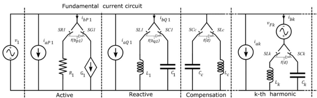
Figure 3:5 Proposed linear equivalent circuit of a generic LED light bulb.
