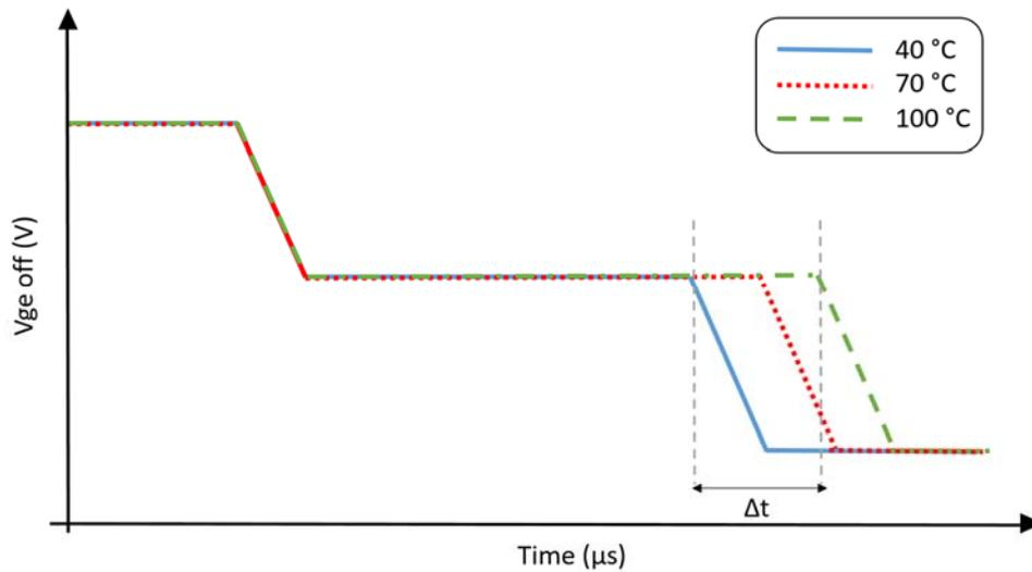
Figure 4:6 Simulated  $V_{ge}$  waveform during the turn off of an IGBT by varying the temperature working operations.
