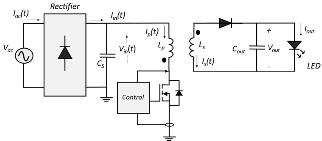
Figure 1:7 QR resonant flyback valley-switching.
