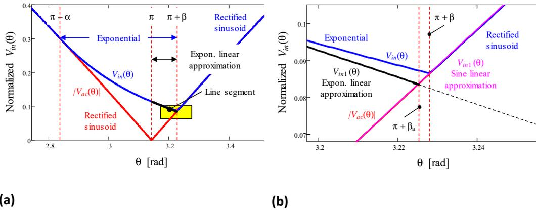
Figure 2:5 Detail of  $V_{ac}(\theta)$  (red trace) and  $V_{in}(\theta)$  (blue trace) near voltage zero-crossing (a), and zoomed view of the yellow area, the intersection of  $V_{ac}(\theta)$  and  $V_{in}(\theta)$  (b). Values are normalized to  $V_{PK}$ .
