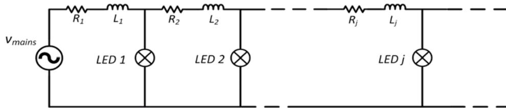
Figure 3:31. Circuit to simulate the current of the overall lighting system.
