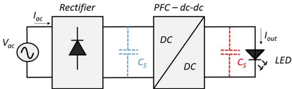
Figure 1:4 Switching -mode single-stage driver: depending on the position of the capacitor  $C_s$  the single dc-dc converter can provide both PFC and output current regulation.
