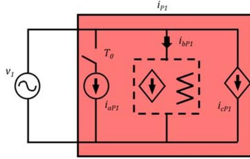
Figure 3:21 Equivalent circuit for the active current. Only one element in the dashed box has to be used (it depends on the sign of  $b_{p1}$ ).
