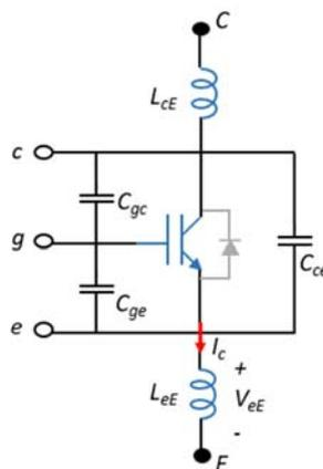
Figure 4:8 IGBT module equivalent circuit.
