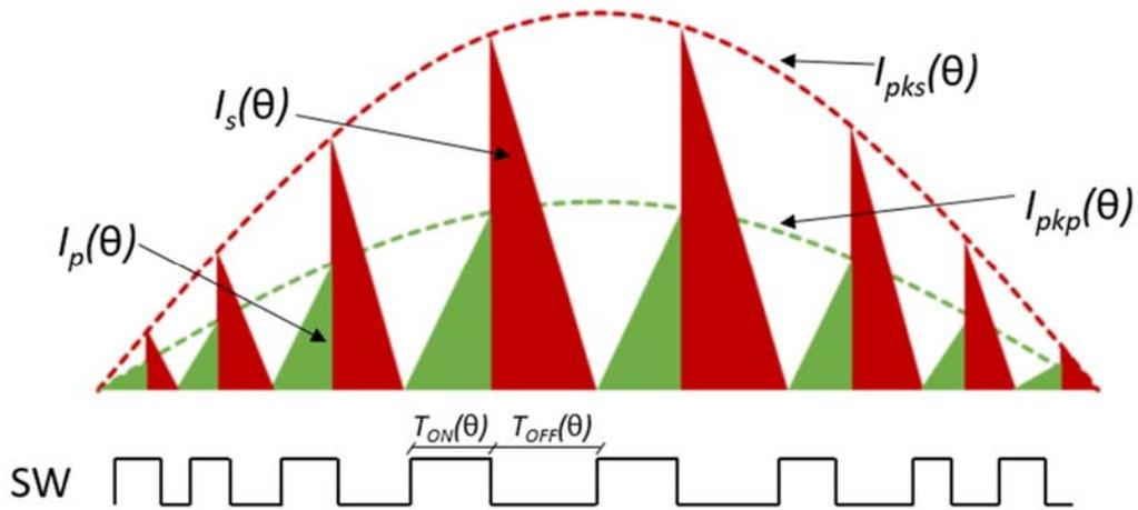
Figure 2:1 Primary and secondary currents in a QR-controlled Hi-PF flyback converter.
