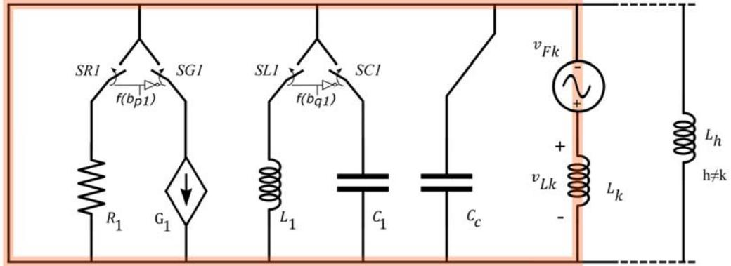
Figure 3:6 Equivalent circuit when only  $v_{Fk}$  works while the other independent generators are turned off. It is apparent that this generator supplies only  $L_k$ .
