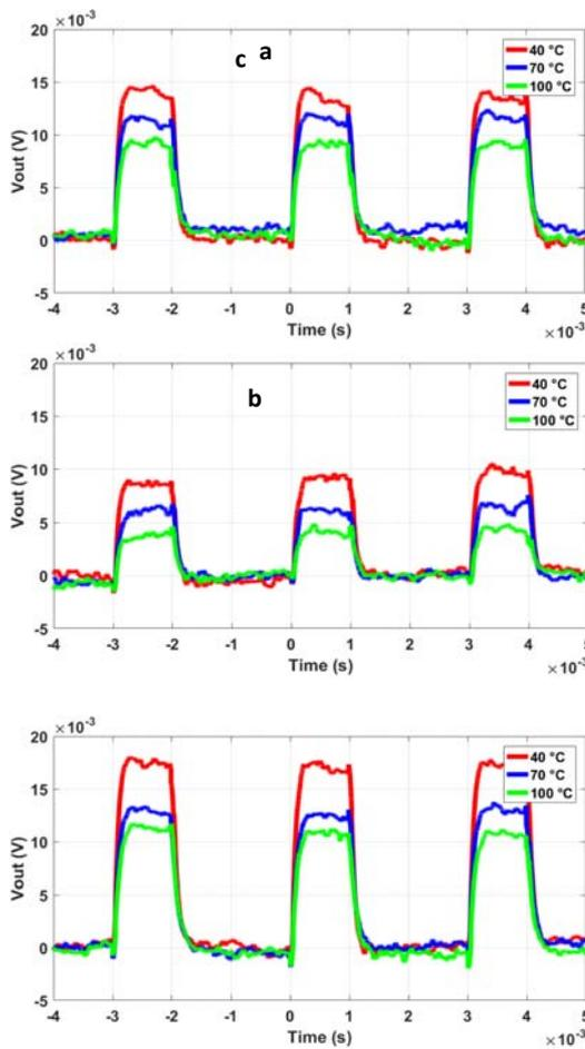
Figure 5:4 Photodiode voltage output at different  $T_j$  and different diode forward current values: (a)  $I_L = 4,5A$  (b)  $I_L = 7,5 A$  (c)  $I_L = 11,5 A$ .
