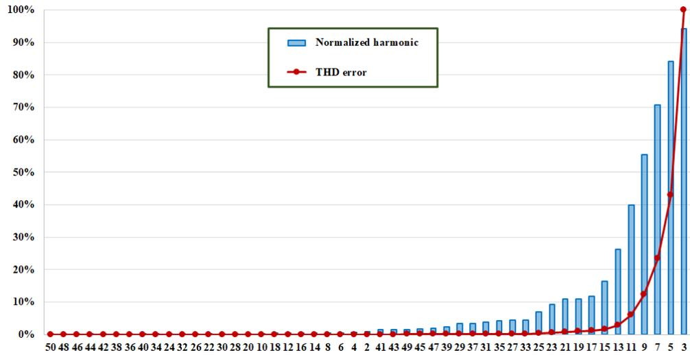
Figure 3:4 Normalized current harmonics and THD error, when the LED light bulb is feed with 237V.
