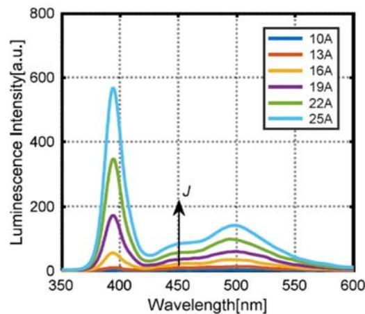
Figure 5:1 Luminescence intensity under different forward currents at 120 °C. (spectrum adopted from [221]).
