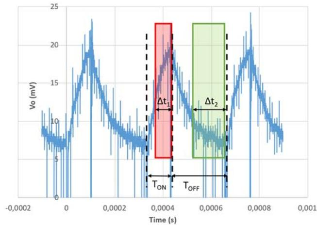
Figure 5:6 Experimental photodiode voltage output at  $T_j = 40$  °C with a  $I_L = 11,5$  A at 3 kHz. Both the subinterval  $\Delta t_1$  and  $\Delta t_2$  represent the last 30% of the  $T_{on}$  and  $T_{off}$  time.
