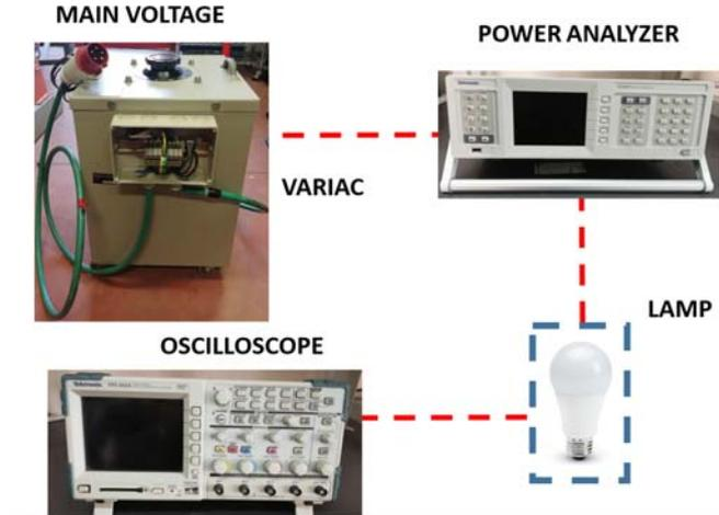
Figure 3:2 Experimental setup. A variac, connected to the mains, feeds the LED light bulb through a power analyzer that acquires the measurements. The oscilloscope displays the waveforms.
