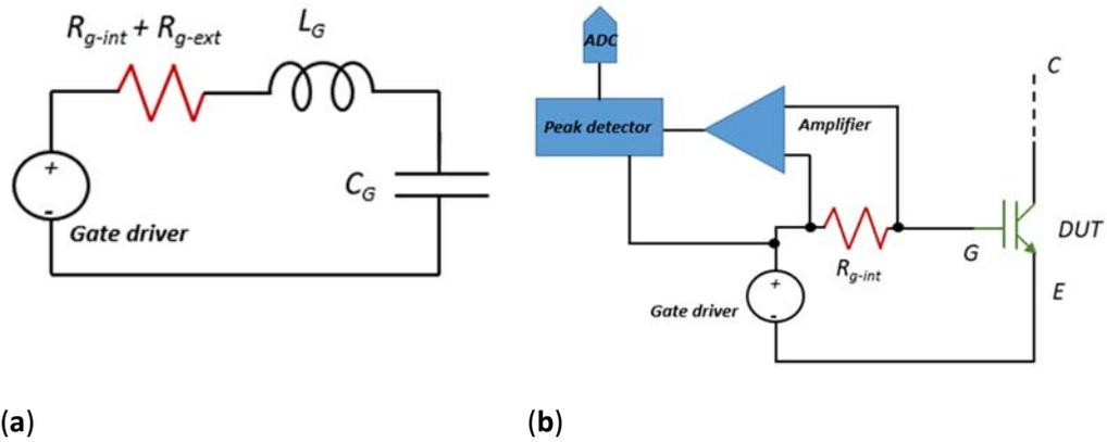
Figure 4:9 Gate driver RLC network. (a) Peak Detector Schematic to detect peak voltage over the external gate resistor.
