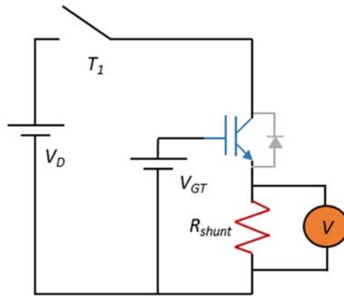
Figure 4:4 Electrical circuits for the measurement of the saturation current in an IGBT device.
