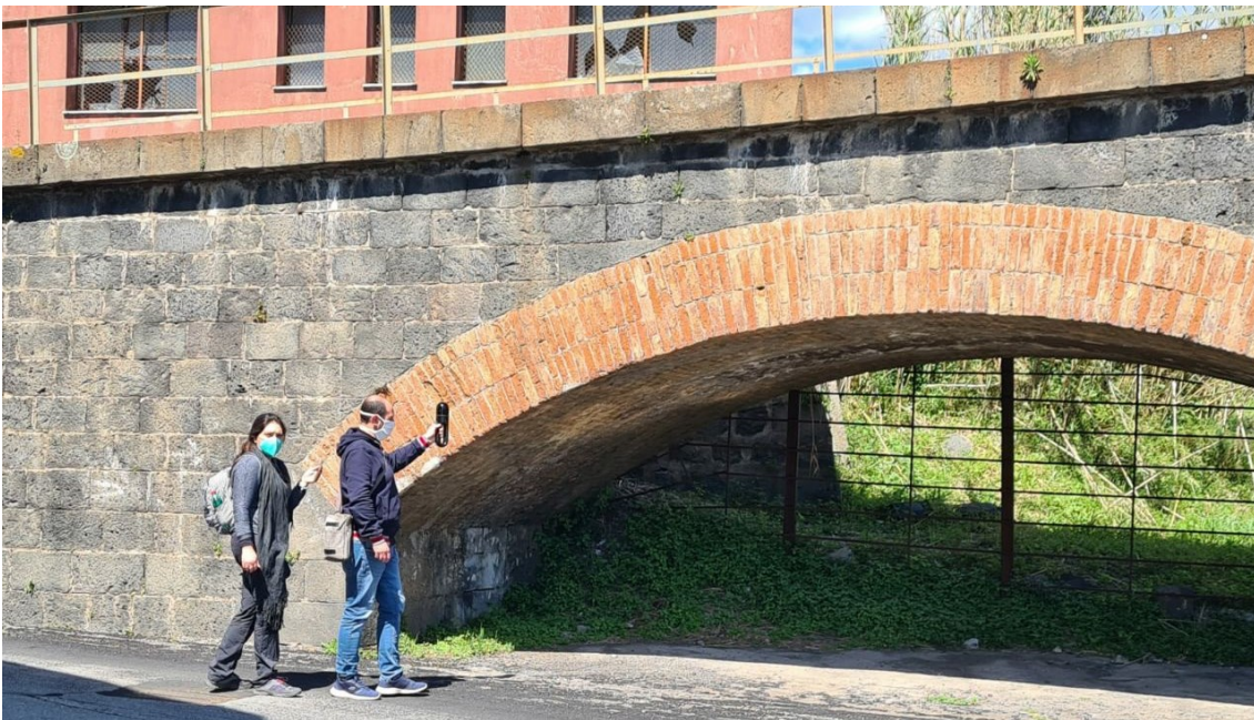
Figure 18 The bridge survey using the BGLK2GO
