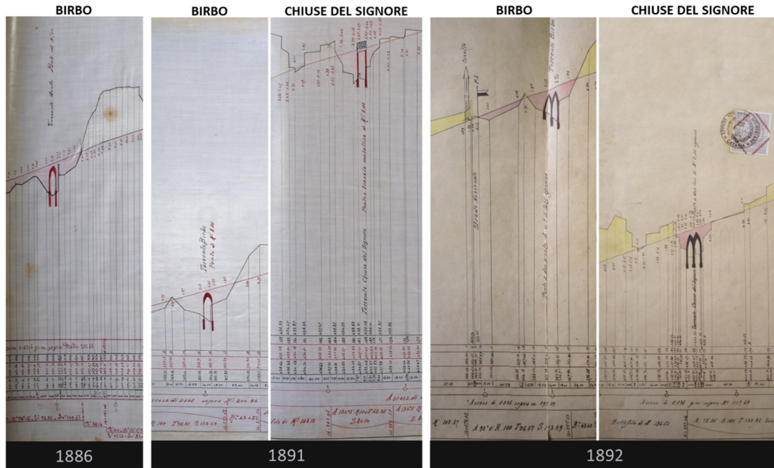
Figure 12 - Longitudinal profiles of the line in correspondence with the bridges over the Birbo and Chiuse del Signore rivers
