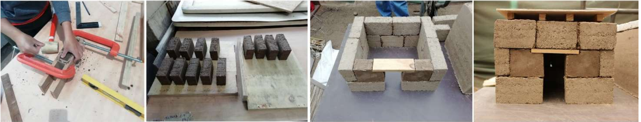
The construction of the concrete-reinforced rammed earth prototype
