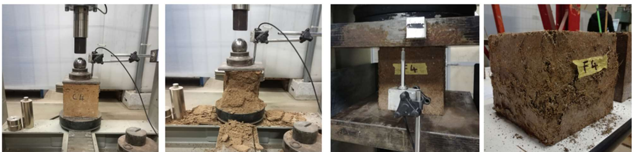
Figure 14 – Compressive behavior of the second-generation batches.
