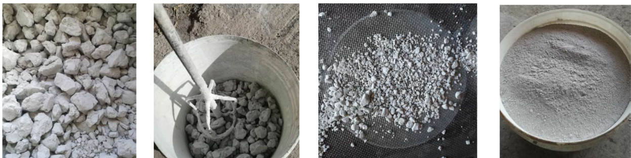
Figure 8 – The dried material is mixed and then sieved in diameters < 2 mm (Daniele Calderoni, 2019)
