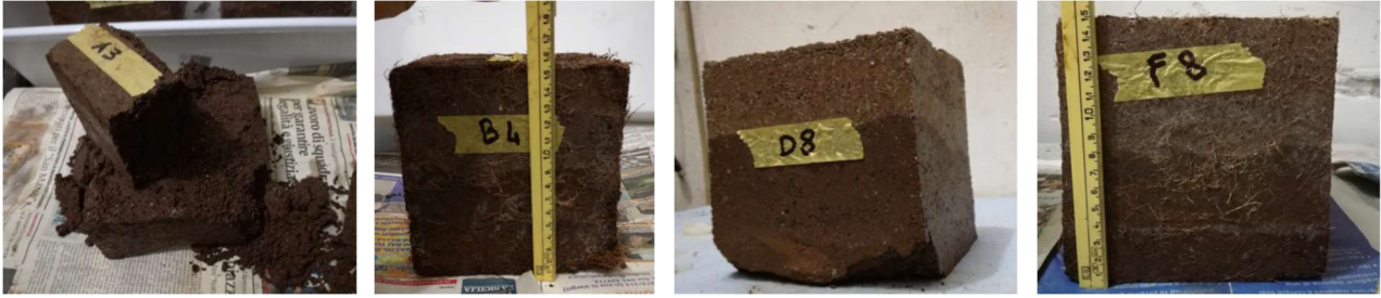
Figure 17 - Different batches at the end of the absorption test
