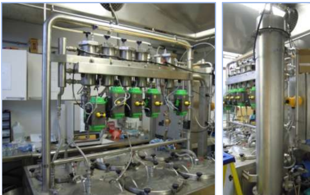
Figure 2.2.1. Two stage UASB reactor. On the left hydrolysis part, on the right methanogenesis part
