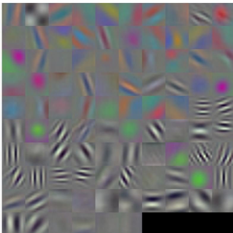
Figure 3.29: First Convolutional Layer weights
