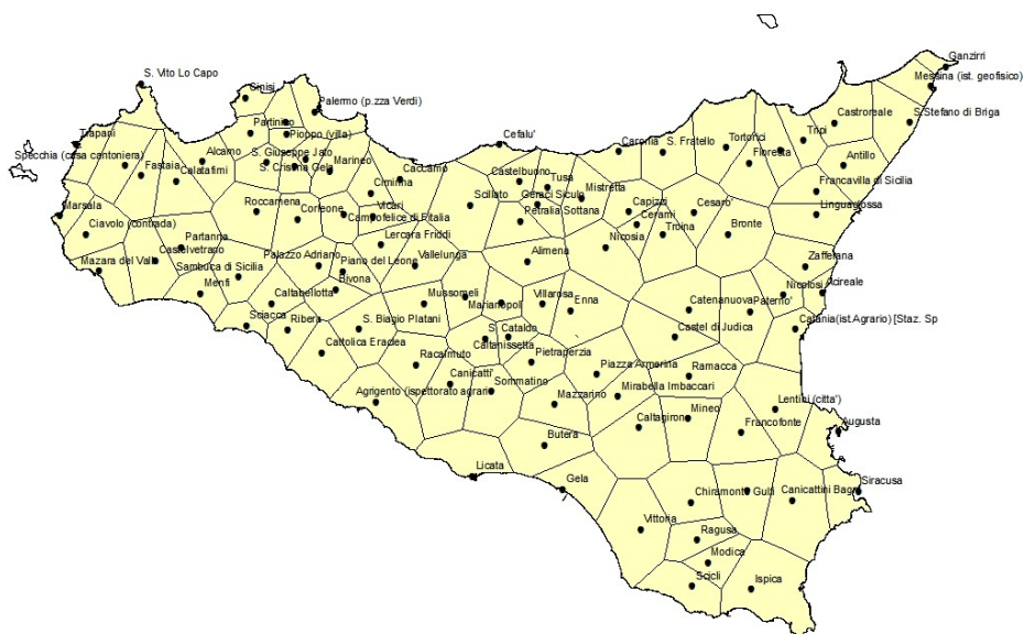
Figure 4.3 – Thiessen polygons associated to each selected rain station.
