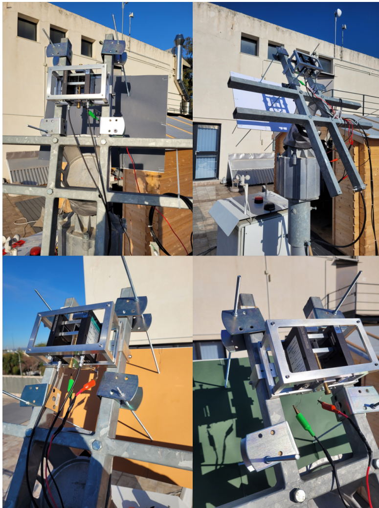
Figure 4.8: Pictures of the P2T device mounted on the bi-axial solar tracker with a gray, white, orange and green paper sheet.
