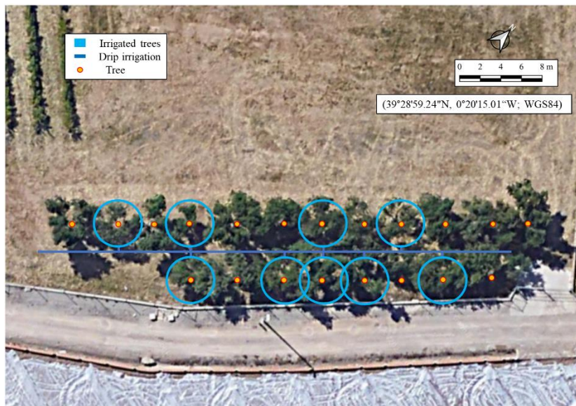
Figure 92. Experimentation site location and irrigation design. Blue lines represent the drip irrigation system used to apply the full irrigation (FI) treatment.
