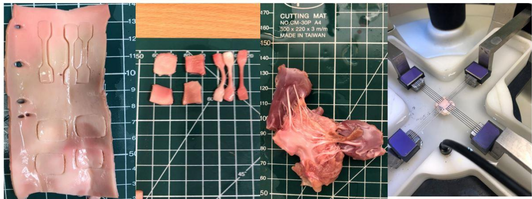
Figure 10 In this figure it is possible to identify the preparation of the specimens of the various monoaxial and biaxial tests and in particular an extraction of a valve with the relative tendon cords is shown. Finally, the arrangement of the specimen inside the biaxial test machine.
