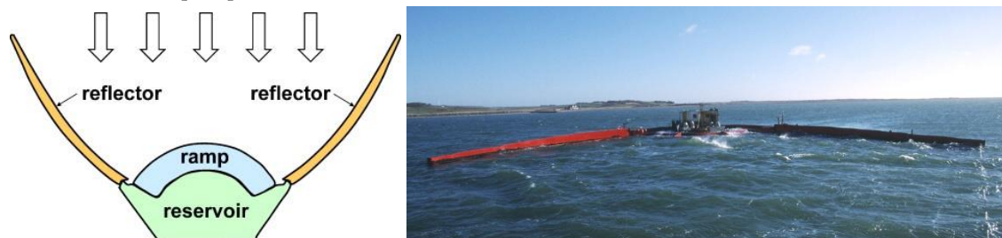
Figure III.29 Views of the small scale Wave dragon (left) [151] and its working principle (right) [189] (Elsevier license n. 4707220104485 and 4707240446626)
