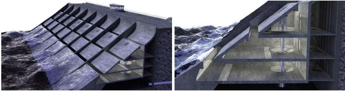
Figure III.30 External view (left) [134] and section view (right) [190] of Slot-Cone (CC BY 4.0).
