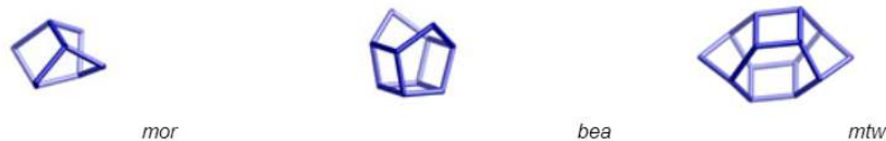
Figure 1.7: The three composite building units in which the BEA framework can be deconstructed, from the International Zeolite Association [51].
