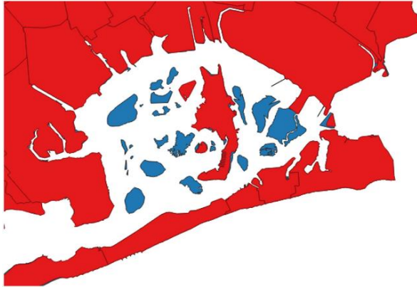
Figure 6.1: example of geometric inconsistency. Even if they are supposed to represent the same spatial subdivision, the polygons of the red layer do not match the polygons of the blue layer, that contains several islands that are inexistent in the red layer.
