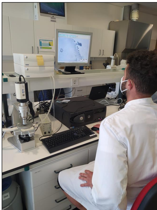
Figure 7 Microthermometric analysis of fluid inclusions conducted at the laboratory of the Instituto de Investigação em Vulcanologia e Avaliação de Riscos (IVAR), Ponta Delgada, Portugal. In the picture, the Linkam MDSG600 heating-cooling stage.
