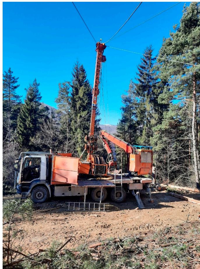
Figure 2. Syncrofalke 3t Processor Tower Yarder.
