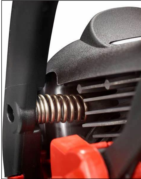
Figure 3 - Anti-Vibration (AV) system in chainsaw
