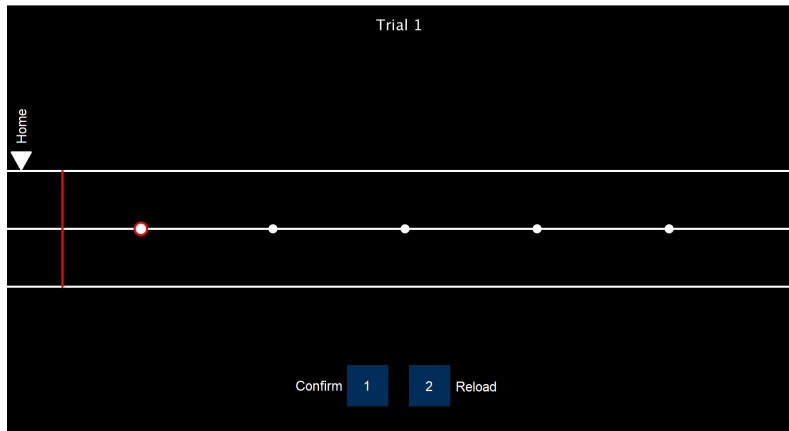
Figure 4.3: The GUI used in the experiment. A vertical red cursor is controlled by the haptic knob; it moves along a virtual horizontal slider which hosts five round markers. At each trial, one marker is highlighted with the red color, thus becoming the current target. The blue squares are activated by pressing the corresponding buttons on the computer keyboard.
