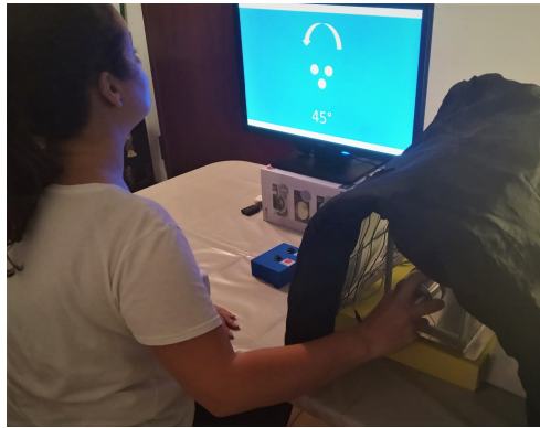
Figure 5.3: Participant grasping the cylinder of the finger tracker while reading the rotation to be performed ( 45^\circ counterclockwise in the represented case).
