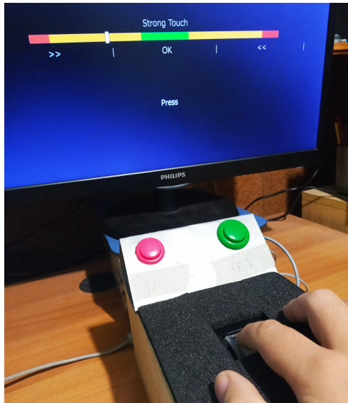
Figure 3.9: Experiment setup: a subject pressing on top of the actuated element while the coloured bar displays the target force.
