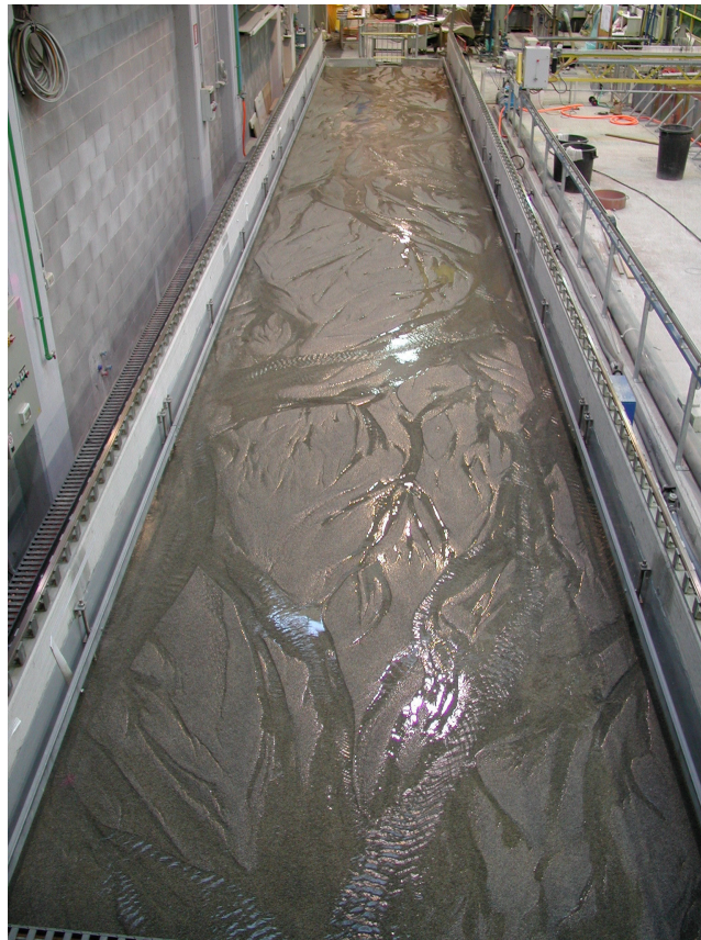
Figure 4.7: Picture of the flume during W3 C5 ( W = 2.9\text{ m} ). Flow is from the camera, discharge is Q = 1.5\text{ l/s} .
