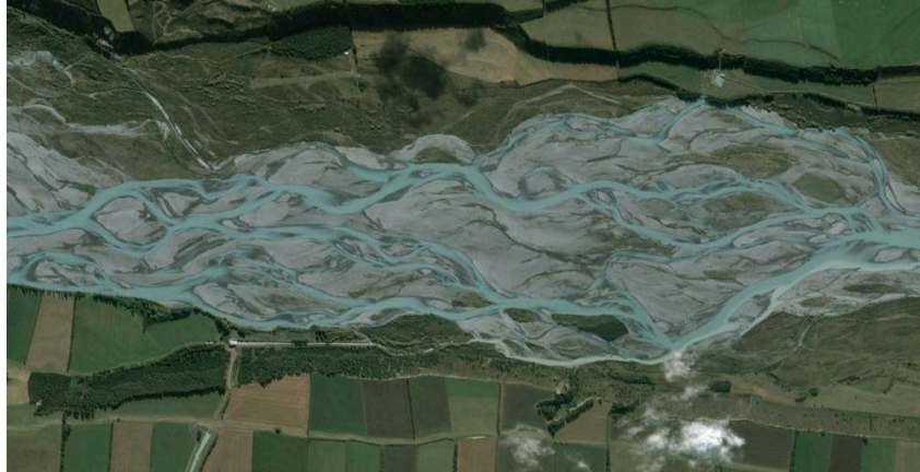
Figure 8.1: Braided reach of the River Rakaia (New Zealand, 43^{\circ}34' S , 171^{\circ}45' E ); from Google Earth, Digital Globe (2014) . Flow is from left to right.
