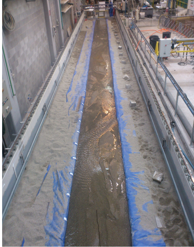
Figure 4.5: Picture of the flume during experiment W1 ( W = 1\text{ m} ). Flow is from the camera, discharge is Q = 2.0\text{ l/s} .
