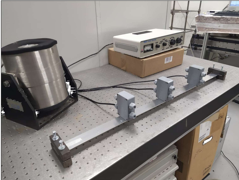
Figure 23: Metal bar excited by white noise.
