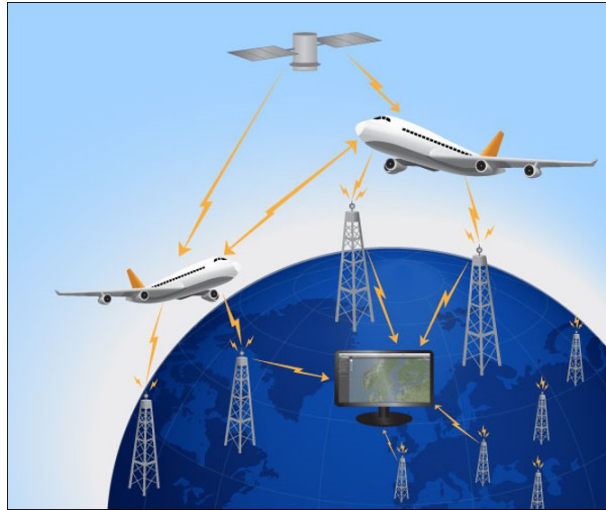
Figure 3.1: ADS-B surveillance technique for Air Traffic Control
