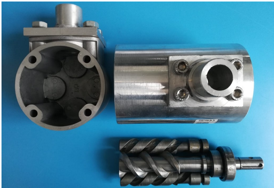
Figure 4-8. Standard triple-screw pump considered for the model validation, disassembled to show driver and idler screws.
