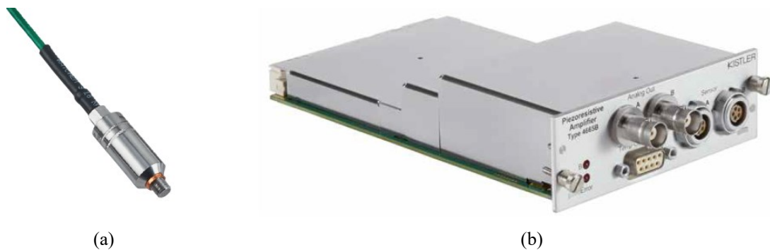
Figure 7-2. Piezoresistive pressure sensor installed on the pump case (a), and Kistler™ signal conditioning system (b).
