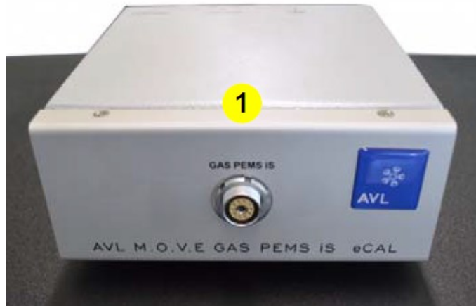
Figure 8-39. AVL eCAL module for the calibration of the AVL GAS PEMS is+ [277].
