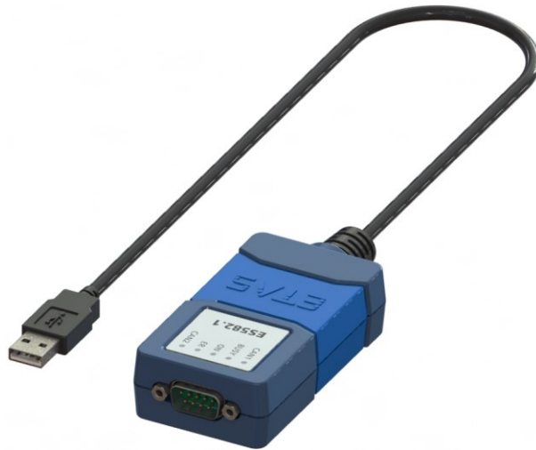
Figure 8-21. ETAS ES582.1 stand-alone module, with an USB port and a CAN FD Bus Interface [275].
