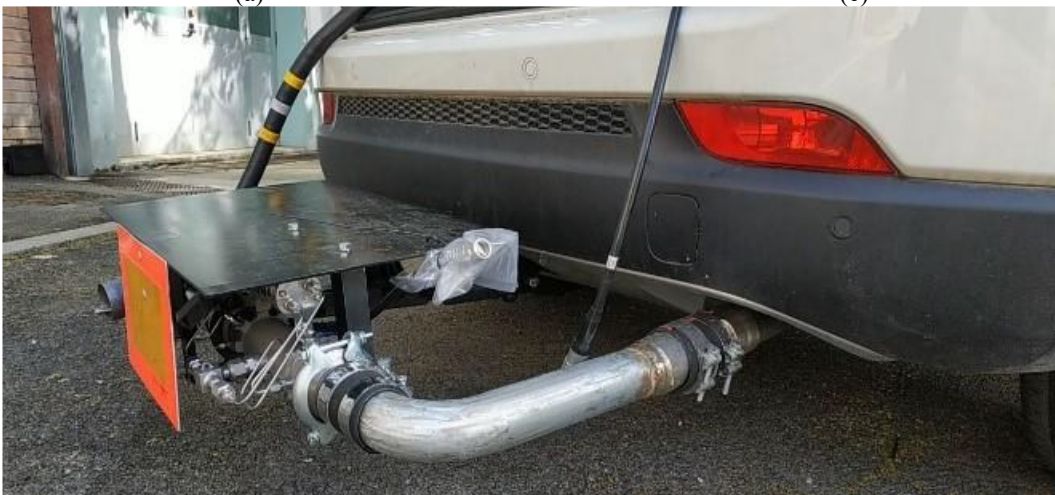
Figure 8-32. AVL M.O.V.E EFM: flow meter (a) installed along the engine exhaust line (b), and control box (c).
