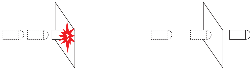
Figure 4.2. An example of what happens when the collisions are only checked at discrete steps and not continuously: a bullet moving at a velocity significantly higher than the framerate, such that the displacement of the object between two frames is larger than the object size, will pass through a thin geometry without registering collision.
