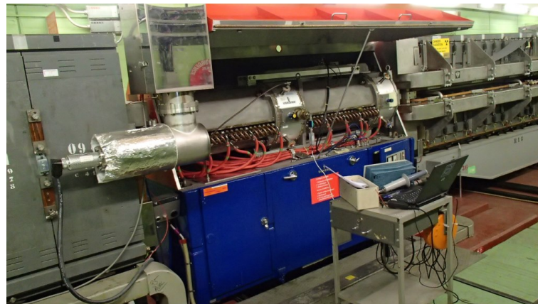
Figure 2.10. One of the accelerating radio frequency cavities of the 10MHz system. The actual ferrite loaded tunable cavity is in the top, under the red hatch. The blue base contains the power amplifiers.
